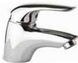
SAGA basin mixer WELS 4 Star, 7.5 ltr/min Reach: 110mm Clearance: 40mm 40mm Cartridge
